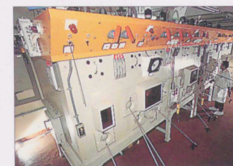
Freeze-drying of pharmaceutical kits in aseptic conditions of a Clean Room
