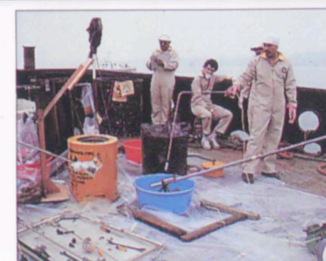
Use of radiotracer in sediment transport studies at Bintulu Port
