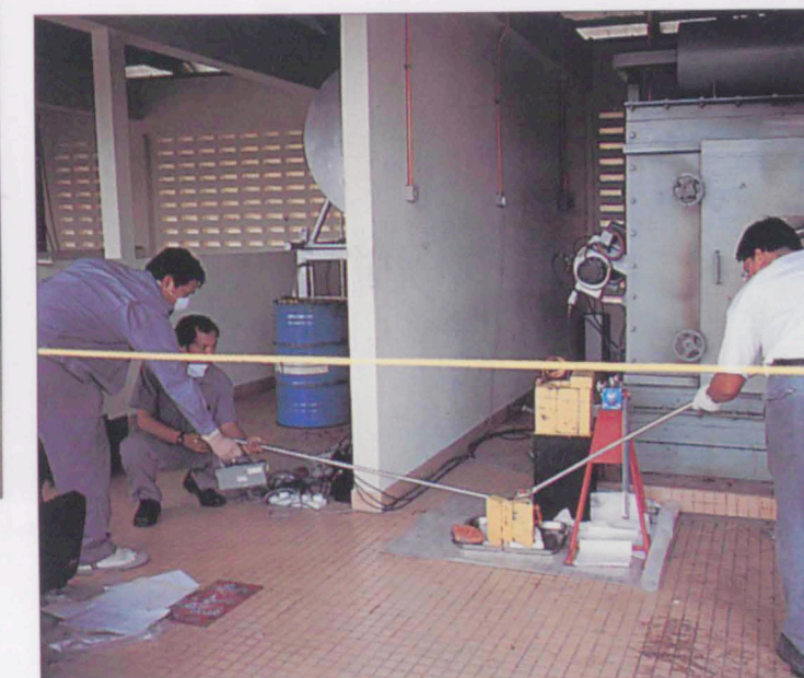
Using radiotracers in studying the efficiency of industrial incinerators
